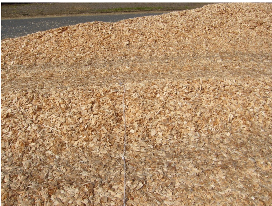
Figure 10 - Compaction of wood chip after wheeled dozer had run over wood chip
