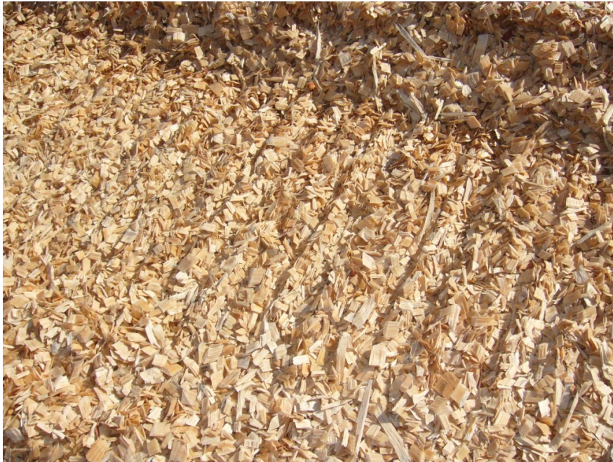
Figure 9 Track Dozer "fluffed" chip after machine had run over wood chip
