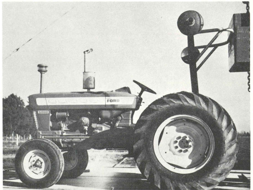
Safe "T" safety frame after impact from rear.
