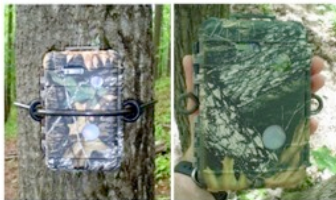
Figure 6. DigitalEye camera traps in their waterproof casing and attached to a tree (Photos courtesy of PixController Inc, DigitalEye™ Trail Camera)
