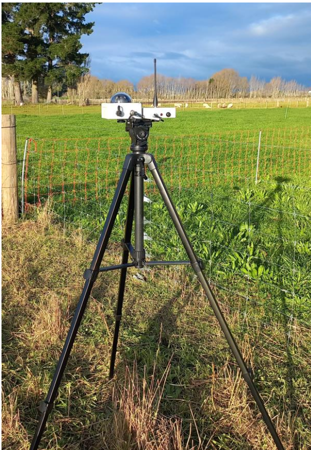
Figure 3.5: Sunshine Sensor (left) and radio link (right) of the SunScan.
