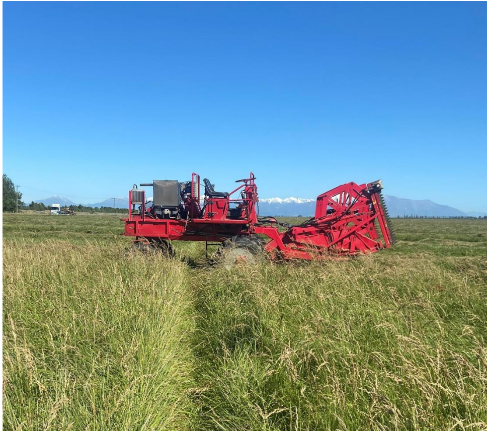
Figure 7. Wintersteiger plot windrower used for trial.
