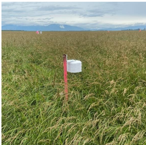
Figure 5. HOBO MX2301A datalogger weather station with a MX2300 Large Solar Radiation shield out in the field.
