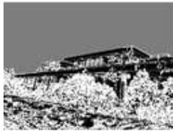
Figure 8: The result of the image after applying a FloodFill algorithm to the upper region in Figure 6 (c). The grey colour represents the sky.
