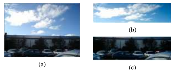
Figure 3: The original colour image (a) is separated into sky region (b) and non sky region (c).
