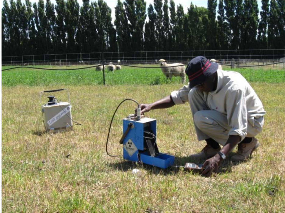
Plate 1 Neutron Probe and TDR used for soil moisture measurements.
