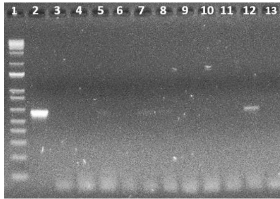
Figure A.11.4: Reaction #55: A product approximately 650 bp of a Cox2 loci was amplified during PCR using primers, Cox2-F and Cox2-RC4 , from samples of dehydrated field pods (S1 samples). Bands indicate the presence of Peronospora viciae f. sp. pisi . Lane 1: 1 kb+ ladder. Lane 2: positive control. Lane 13: negative control. Lanes 3-12: Dehydrated field pods from Site 1, Plant 1.
