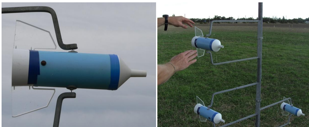
Figure 6.6 Leuning NH 3 sampler(s) on the mast.
