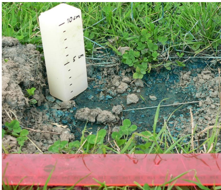
Figure 6.5 Photo of urine patch size simulation using brilliant-blue dye in aqueous solution.
