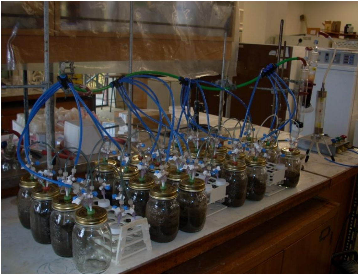
Figure 7.1 Photo of the incubation jars, during experiment 1, connected to the incoming \text{NH}_3 scrubbed air and the downstream acid traps for capturing \text{NH}_3 volatilised from the incubation jars. Note empty jar, one of two run as experimental blanks.
