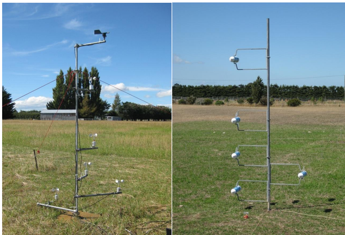
Figure 6.3 Photos of wind profile (left) and NH 3 profile (right) masts.
