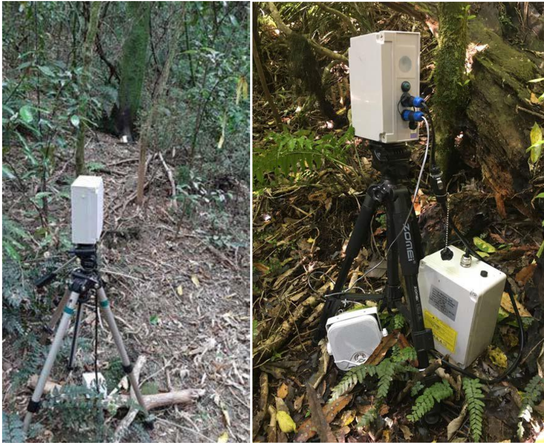
Figure 3.6. Example of experimental set up at Living Springs (left). Thermal camera on tripod with battery pack and speaker attached (right) – from trials conducted by Bugler & Ross (2020)
