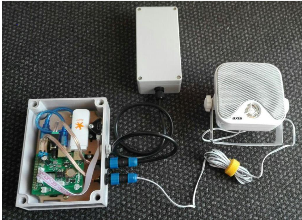
Figure 3.4. Thermal camera interior (left) connected to a lithium battery (centre) and an external speaker (right) (Finlay-Smits, 2018).
