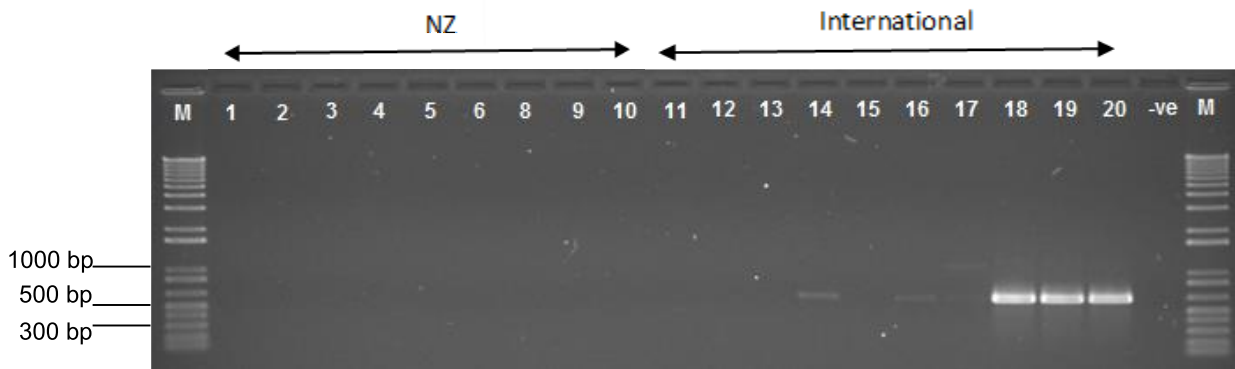
Figure 2.13: 1% agarose gel of PCR products generated by ToxB -specific TB10f and TB12r primers using genomic DNA of New Zealand and international Pyrenophora tritici-repentis single spore isolates. From left to right, lanes 1 to 13 are P. tritici-repentis isolates S12a, S22a, S26a, M13c, M14d, G14a, W12a, W12c, W15a, K16a, CCDM-239, CCDM-134, ASC1, CCDM-Meck4, AB39-2, 90-2, Alg3-24, AlgH2 and TS93-71B. M = 1 kb plus DNA ladder (Invitrogen), - ve = negative control.
