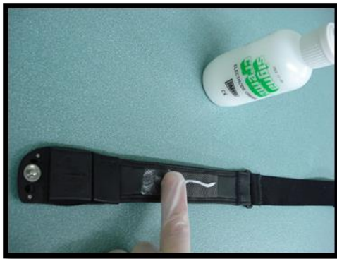
Figure 19: Apply some electrode gel to the electrodes of the HRM belt to improve contact with the skin
