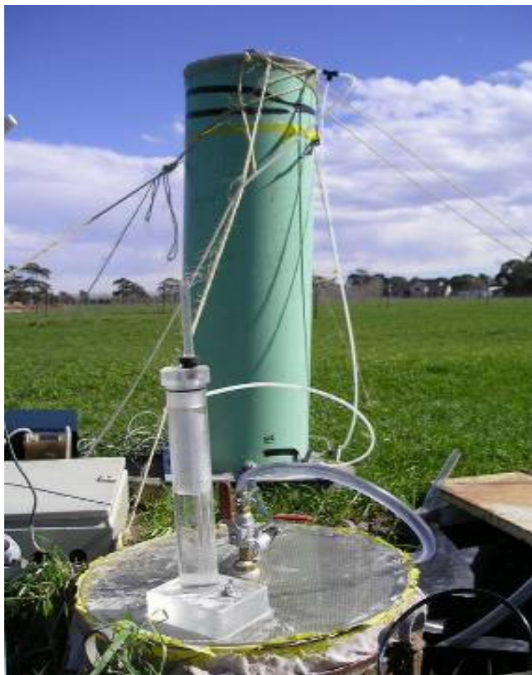
Plate 3.3 Tension infiltrometer apparatus
