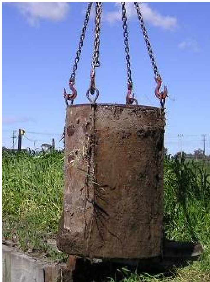
Plate 3.4 Lysimeter being lifted out from side of the trench
