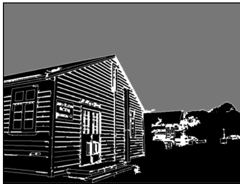
Figure 3.19: The result after applying a FloodFill algorithm to the upper region in Figure 3.18. The grey colour represents the sky.
