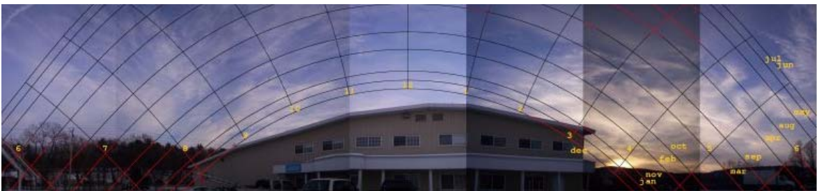
Figure 2.10: Sunpath diagram output by the Acme Solar Site Evaluation Device. The sunpath is shaded red in the non-sky region (Wiley, 2005).
