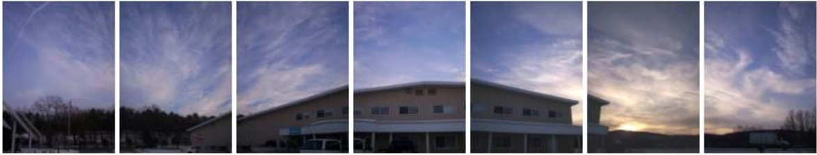
Figure 2.9: A series of 7 pictures for evaluating shading by the Acme Solar Site Evaluation device (Wiley, 2005).
