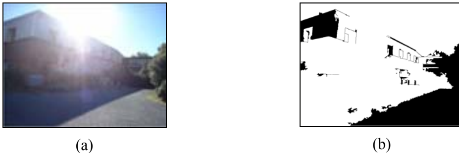
Figure 4.8: Failure of the image processing to correctly identify the sky region. (a) the original image, (b) after image processing.
