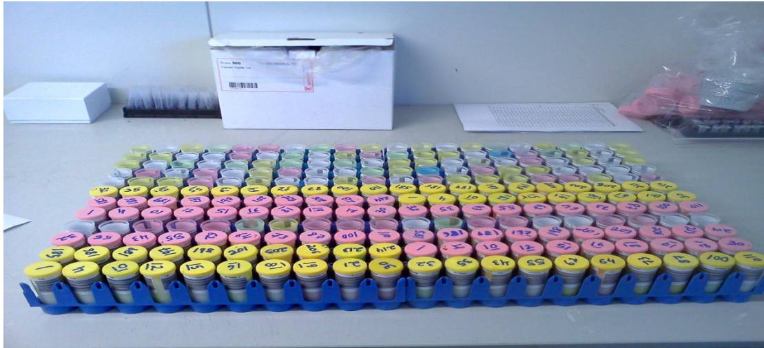
Figure 3.5: Milk samples (yellow = p.m. milking and pink = a.m. milking) packed for analysis of milk composition at Livestock Improvement Corporation Ltd laboratory (Christchurch, New Zealand) to determine milk fat, protein and lactose by Milkoscan™ (Foss Electric, Denmark).
