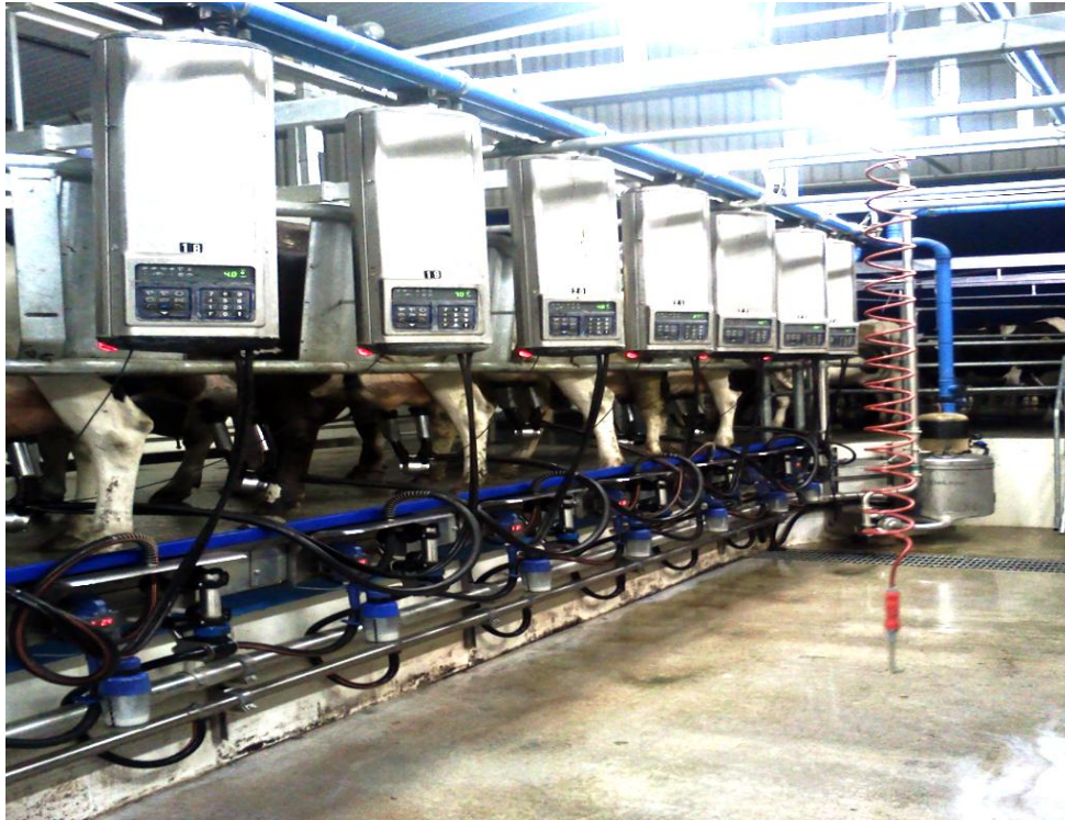
Figure 3.4: Milk subsamples being collected using milk flasks (with blue cover-lids) during a.m. and p.m. milking. Milk yield was also recorded (light green numerals) by the automated system (DeLaval Alpro Herd Management System, DeLaval, Tumba, Sweden)
