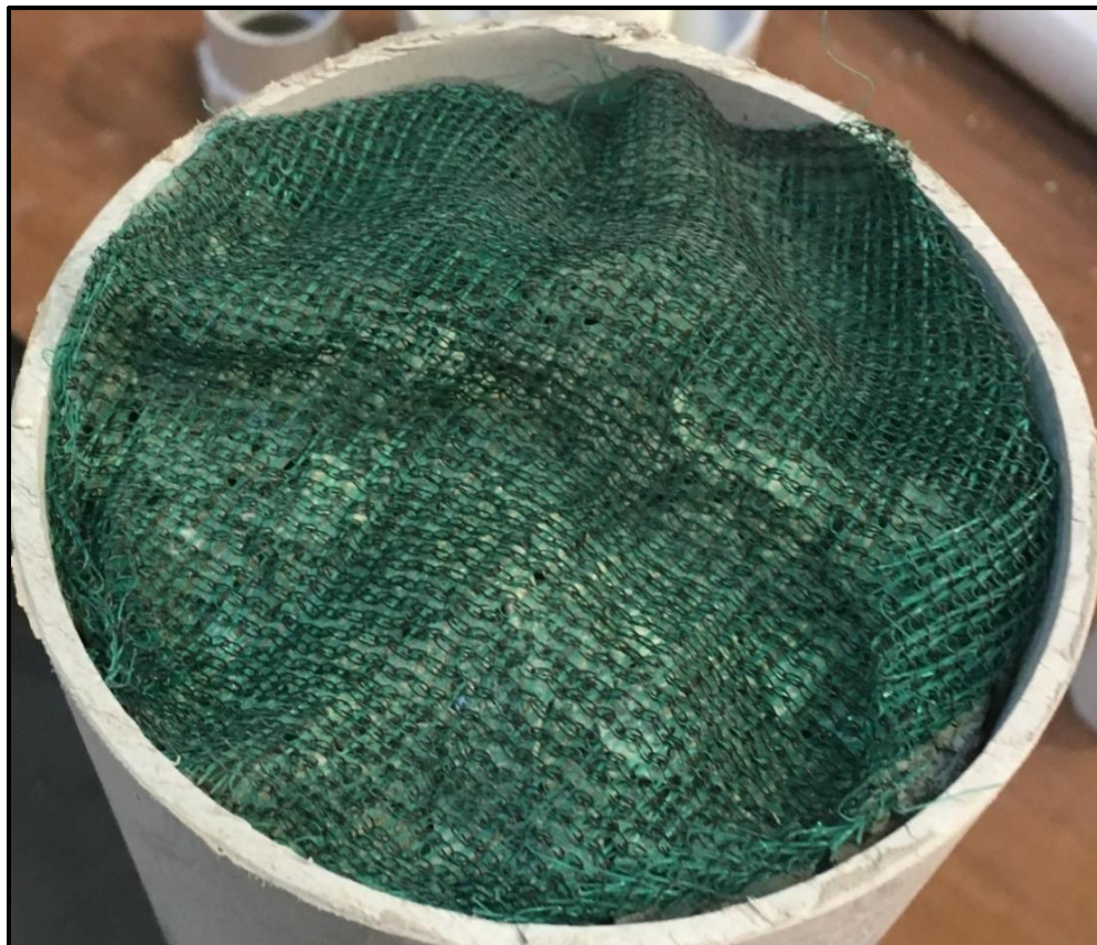
Figure 3.6: The PVC mesh used at the top of each filtration unit to prevent the filtration media being discharged with the overflow through the breathing pipe.
