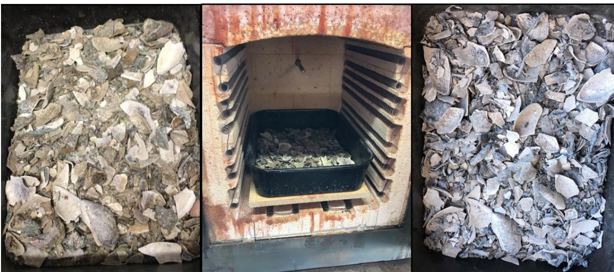
Figure 3.2: The heat treatment of crushed mussel shell: Before - In the oven - After.
