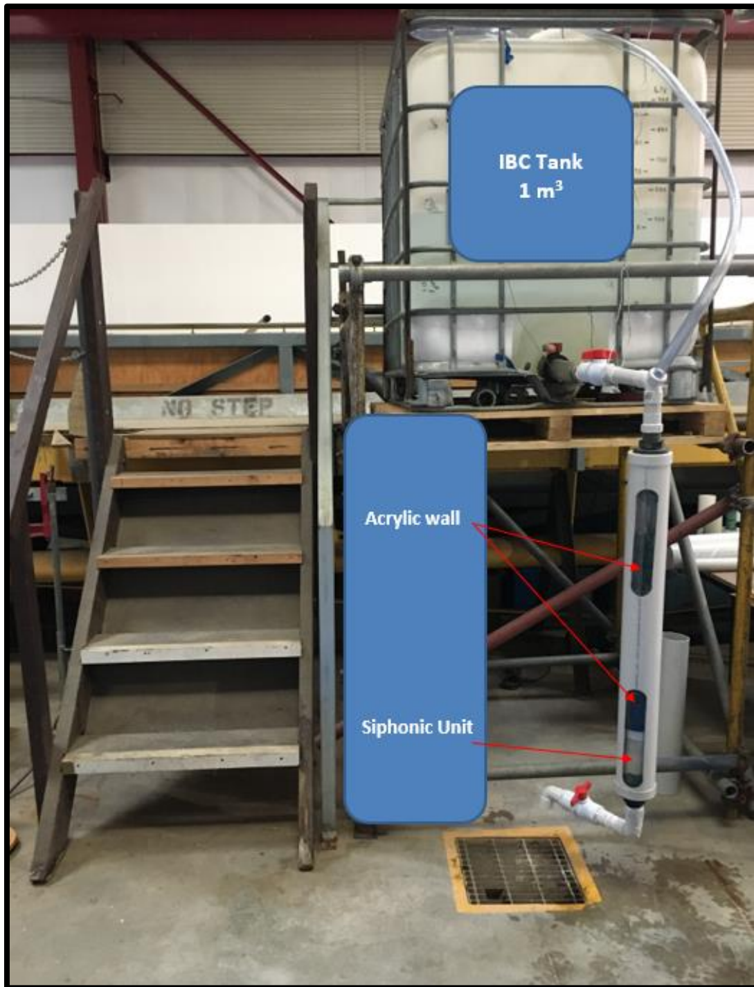
Figure 3.18: The transparent filtration unit which was designed to evaluate the flow patterns through the filtration media during the gravity and the siphonic flow conditions.
