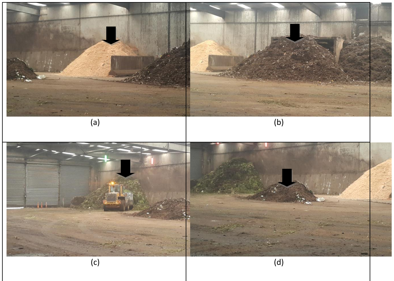
Figure 3.1 waste material ready to be incorporated into compost, a) sawdust; b) partly sorted material that has been brought back in for further composting (tailings); c) unsorted greenwaste d) food waste.
