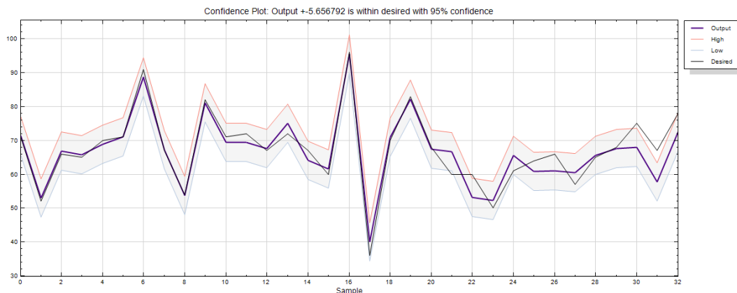
Fig.4. Observed and predicted fuel consumption using an artificial neural network with 95% confidence.
