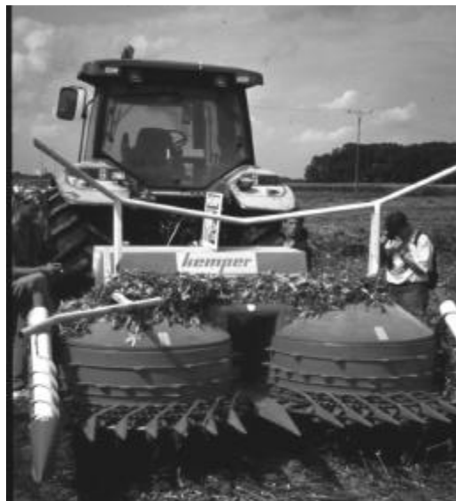
Figure 6. A modern European forage chopper for cutting and windowing hemp (Ehrensing 1998)
